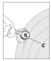
"C", should be turned in a anti clockwise direction until the bolt can be partially withdrawn.
